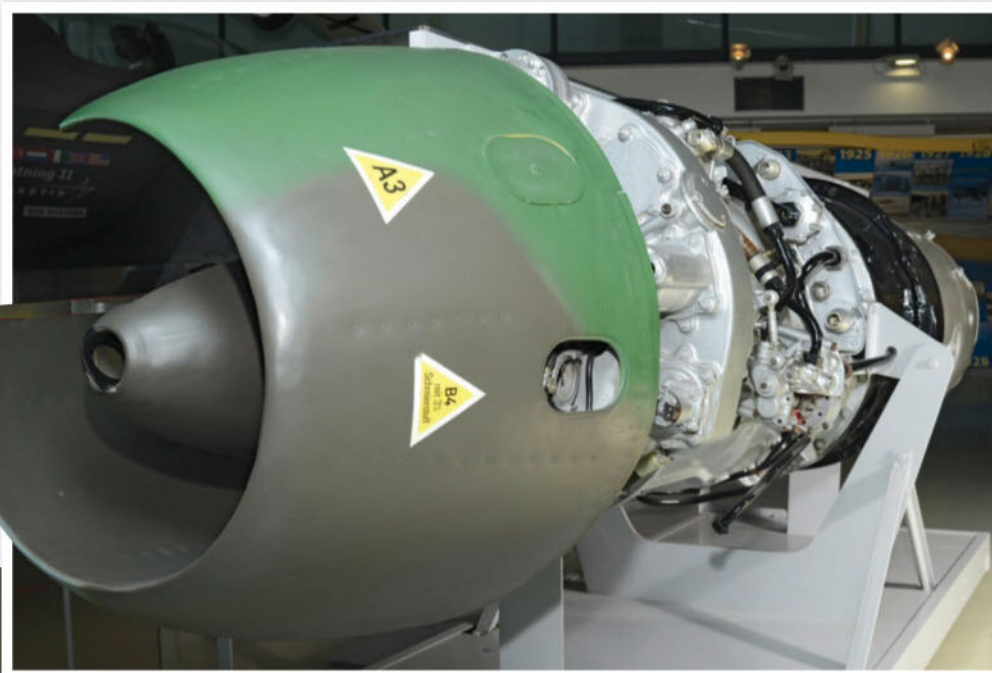
The massive air intake at the forward section of the burly Junkers Jumo 004B engine nacelle directed current through the structure
